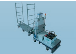
Towing hook type (Motor-powered disconnection type)
